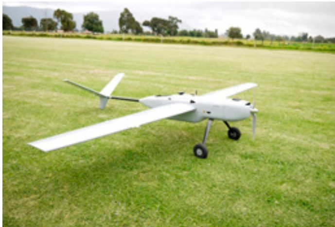
Figure 1. Atmospheric Data Acquisition System ADAS – AQUILA.
